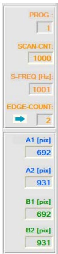
These display elements provide information about the detected edges from the normalised data field. The measurement values for the jet positions, based on the known pixel distances of the receiver line, can be calculated with the following formula:
